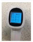
From the off state press and hold trigger button to view first 4 readings
