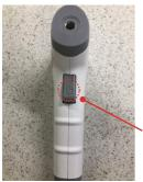
Press the "on" button once quickly and release pressure off the trigger
